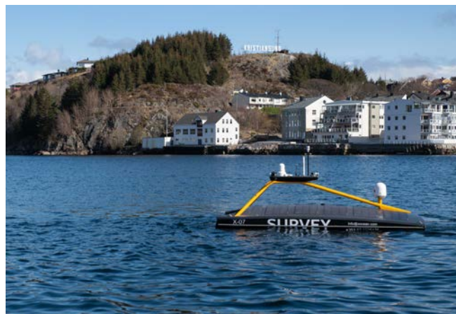
XOCEAN's Sonardyne-equipped XO-450 leaving Kristiansund to harvest data from Sonardyne's Fetch pressure monitoring transponders at Ormen Lange. Photo courtesy of SafePath.
