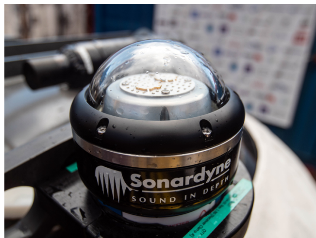
Sonardyne's BlueComm undersea communications system; the only commercial- off-the-shelf (COTS) technology that enables wireless transmission of high bandwidth tactical data, including video, underwater.
