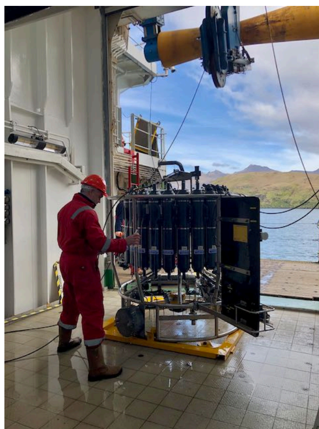
Collecting water samples to calibrate the CTD salinity (photo: A. Marzocchi)
