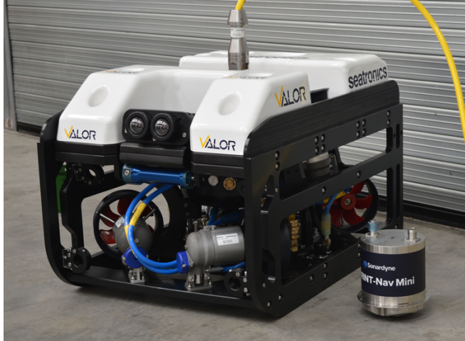
SPRINT-Nav Mini offers both the survey positional accuracy and a small form factor, ideal for small ROVs like the VALOR.
