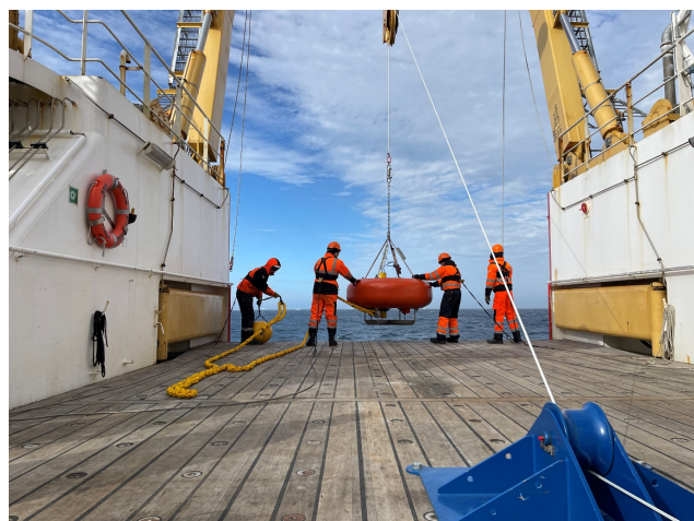
Deploying the top mooring buoy. Photo by Huw Griffiths.
