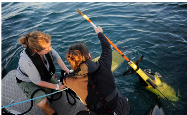
Recovery of a glider vehicle SAMS scientists use to measure temperature and other oceanographic properties in the deep ocean.
