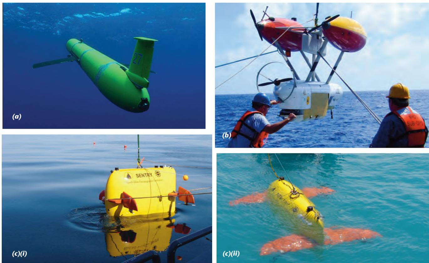
**Figure 2** Examples of some AUVs. (a) A Slocum buoyancy-driven glider. (b) Woods Hole's Autonomous Benthic Explorer (ABE), designed to investigate deep ocean environments such as hydrothermal vents. (c) ABE's successor, Sentry, (i) at the start of deployment, (ii) with its 'glider wings' extended. (Photos by courtesy of: (a) Rutgers University; (b) Dana Yoerger; © WHOI and (c) Chris German; © WHOI)
