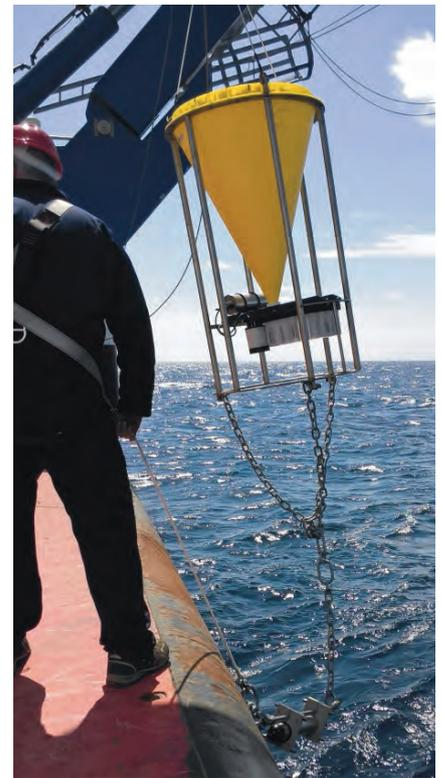
**Figure 4** A sediment trap being deployed at the PAP-SO site. The containers at the bottom move around every 2–4 weeks, allowing each in turn to receive material collected by the funnel, so providing an observational time-series.
