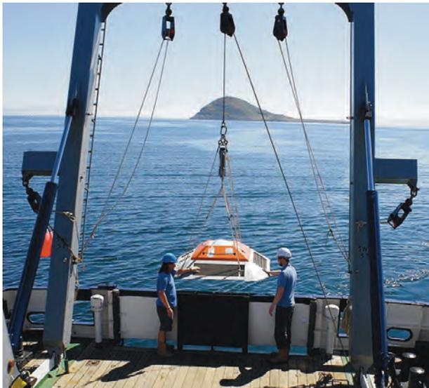
**Figure 2** An ADCP being lowered to the sea bed from the RV Prince Madog. This is part of the range of equipment made available to companies participating in SEACAMS.
