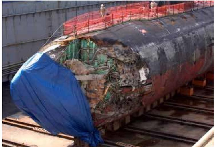
**Figure 9** USS *San Francisco* in Guam in January 2005. The submarine was in collision with an uncharted seamount while travelling at 33 knots between Guam and Brisbane. One sailor was killed and 115 others were injured. (Image source: [https://en.wikipedia.org/wiki/USS\\_San\\_Francisco\\_\(SSN-711\)](https://en.wikipedia.org/wiki/USS_San_Francisco_(SSN-711)).)
