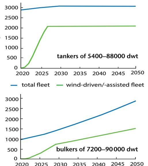
**Figure 6 Predicted increases in the numbers of tankers (top) and bulkers (bottom) making use of wind.** The actual take-up of wind power will depend on the bunker fuel price, the speed of the vessels, and the discount rate applied. dwt = deadweight tonnage, a measure of the total weight a ship can carry. (From a study prepared for the EU by CE Delft 2016)
