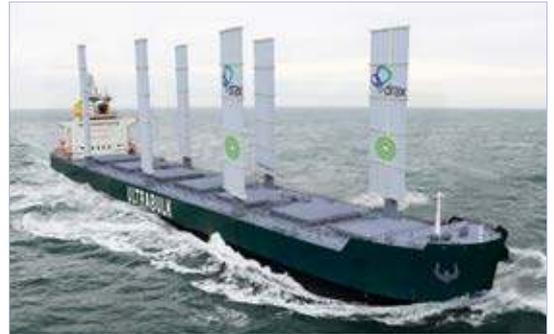
**Figure 2** Examples of rigid wingsail vessels under development.
