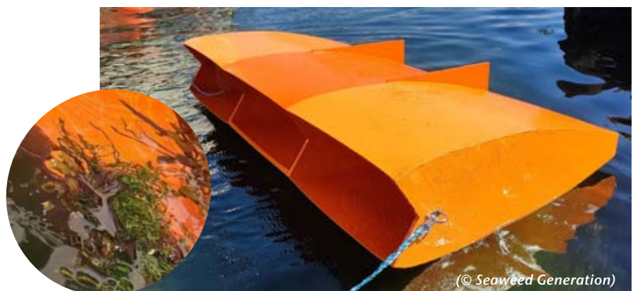
Figure 3 Manta rays cruise for plankton, AlgaRays will scour the surface for Sargassum weed. A prototype AlgaRay is towed behind a boat to tests its performance, but AlgaRay will eventually become fully autonomous. Inset Sargassum being scooped into the AlgaRay.
