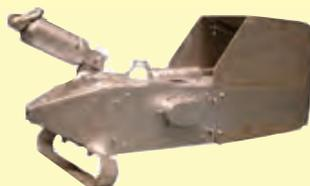
The CPR was originally made of gunmetal (phosphor bronze), but since 1997 has been made of stainless steel. The nose cone is filled with lead. The CPR is towed on a 10 mm diameter wire rope at a depth of about 10 m. It has been operated successfully at speeds of up to 25 knots, and its robust design allows deployment in rough seas. Successful tows have been continued in winds up to storm force 11.
