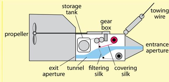
On return to the laboratory, the silk is removed from the cassette and divided into samples (or 'blocks') each representing 10 nautical miles of towing. The plankton on these samples are then analysed according to standard procedures.
