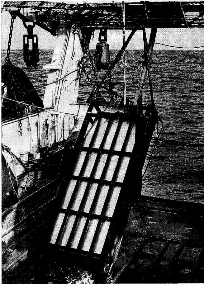
**Figure 2** The 2-m long detritus sledge is emptied onto the deck of the Faroese Fisheries Investigations research ship Magnus Heinason.
