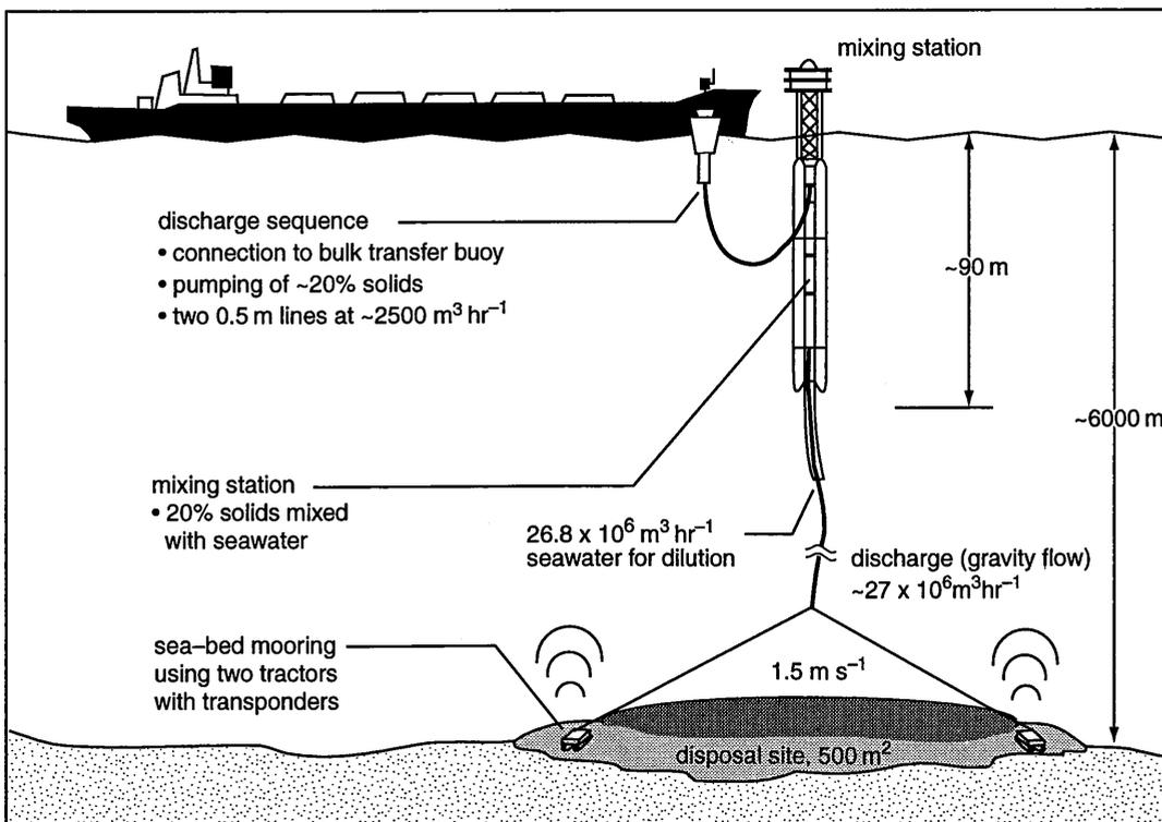
**One possible method for disposing of sewage sludge and dredge spoils in the deep sea**
