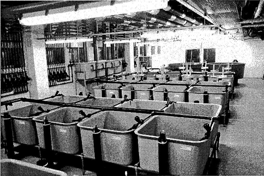
**Figure 3** Fish tanks with water quality and photoperiod control (simulating day-lengths and variations in light intensity appropriate to different latitudes).
