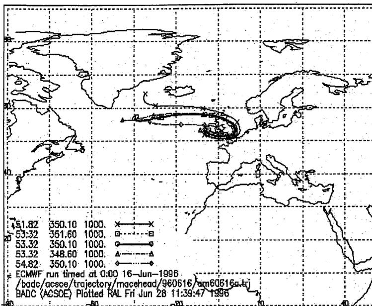
**Figure 7** Five-day air mass back-trajectory for 16 June 1996 (in the middle of the experiment). Northerly winds veer easterly over Scotland and Ireland before arrival at Mace Head and RRS Challenger.
